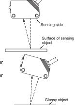
If the sensing object has a glossy surface, however, incline the Sensor by 5° to 10° as shown in the illustration, provided that the Sensor is not influenced by background objects.
