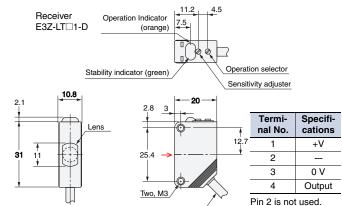
4 dia. vinyl-insulated round cable with 3 conductors (Conductor cross section: 0.2 mm² (AWG24), Insulator diameter: 1.1 mm) Standard length: 2m
