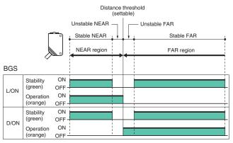
Note: If the stability indicator is lit, the detection/no detection status is stable within the rated ambient operating temperature (-10 to 55°C).
